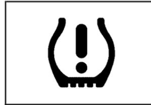
For vehicles with a tire pressure light, this light comes on briefly when the engine is started.
