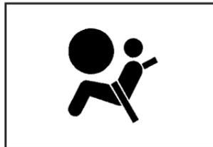
This light comes on when the vehicle is started, and flashes for a few seconds. Then the light should go out. This means the system is ready.
